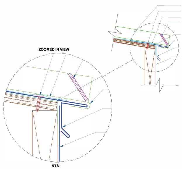
NC 150SS PANEL #10 - 13 x 1" PHW (12" o.c.) NEW CASTLE UNDERLAYMENT NEW CASTLE APPROVED TUBE SEALANT (FIELD APPLIED BETWEEN PANEL RIBS) NEW CASTLE UNDERLAYMENT FIELD CUT & HEM PANEL 180°
