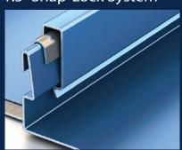
The NC550S is a concealed fastened snap lock system with an integral locking panel. This means the panel is securely engaged along the entirety of the rib. Our most popular residential panel, can be installed quickly without sacrificing quality.
